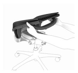
35. Lift up front of seat assembly and remove.
