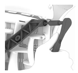
18. Remove the two top antler attachment screws using a T-27 torx wrench.
