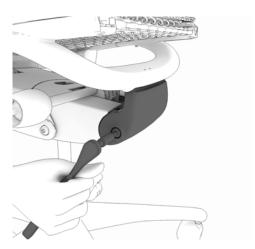
33. Remove two lower front link shoulder bolts and bushings using T-40 torx wrench.
