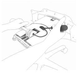
36. Locate wire clip for tilt tension knob. Slide flat blade screwdriver under cable collar. Pry up gently until cable collar is free.
