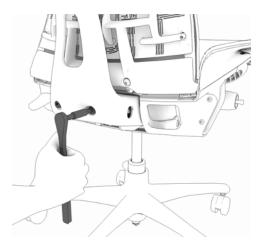
9. Remove both lower spine bolts using T-40 torx wrench.
