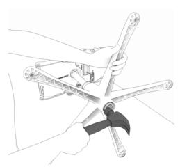
49. Hold base legs firmly and strike the bottom of cylinder with a 2 pound hammer until base comes loose.
