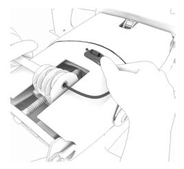
37. Grasp the cable and push it forward to release ball end from cylinder.
