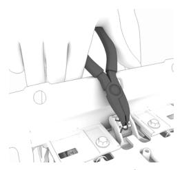
42. Remove wire clip from tilt tension knob assembly.
