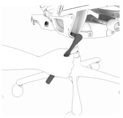
32. Remove single lower bolt from each arm housing using T-27 torx wrench. Repeat for opposite side.
