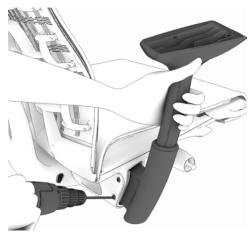
4. Remove both bolts using power driver to remove arm. Repeat for opposite side.
