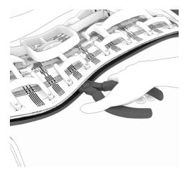
13. Insert needlenose plier between fabric and wiffle material. Twist plier until attachment pegs pop loose. Repeat for all pegs.
