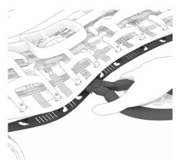
23. Insert needlenose plier between back strap and twist plier until attachment loose.
