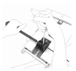
38. Hold the Knob assembly using a flat blade screw driver. Pull the tension knob using other hand.
