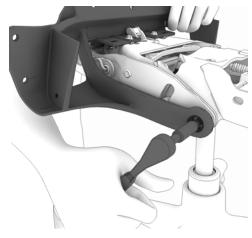
44. Remove shoulder bolt and flange bushing from each side of rack.
