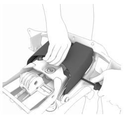
40. Slide flat blade screwdriver along side of rear tilt cover and pry off.
