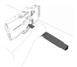
52. Pull out the cylinder from assembly.
