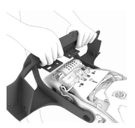
46. Rotate rack and pull free from assembly.
