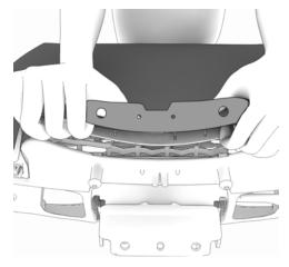
26. Disengage the fabric from rear mount posts.
