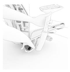
3. Pull to remove back angle adjust handle.
