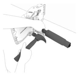
51. Hit the bottom of the chair with hammer until cylinder separates from chair.
