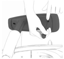
1. Remove front and back screws of arm pad using T-20 torx driver.
